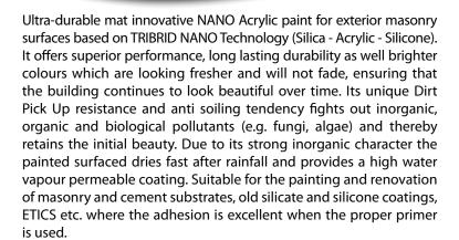
Acrylan MAX based on tri-hybrid nanotechnology combines all the advantages of silicate, acrylic and silicone paints, offering very high added value to the buildings due to lower renovation cost and longer lifetime as well as very low environmental impact.
